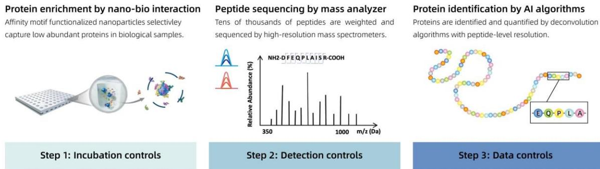
**Figure 2.** Quality controls in Proteonano™ Platform with signal readout by mass spectrometry.
