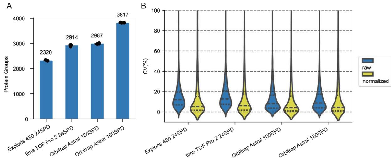
**Figure 9.** Comparison of performance of Proteonano™ platform on different mass spectrometers. (A) Number of protein groups identified in detected by different mass spectrometers. Bar height, and number indicate mean protein groups detected in each mass spectrometer. Individual dots represent protein groups detected in each MS run. (B) Distribution of CV values of protein intensity among different mass spectrometers.
