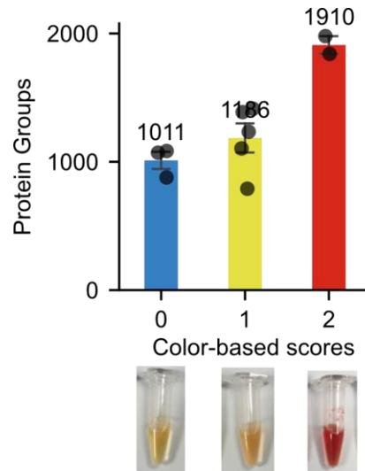
**Figure 10.** Detection depth of samples with various levels of hemolysis. Samples were processed by the Proteonano™ platform and analyzed by a timsTOF Pro2 mass spectrometer.
