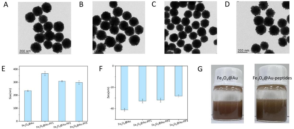
**Figure S2.** TEM images of  $\text{Fe}_3\text{O}_4@Au$  (A),  $\text{Fe}_3\text{O}_4@Au\text{-PP1}$  (B),  $\text{Fe}_3\text{O}_4@Au\text{-PP2}$  (C) and  $\text{Fe}_3\text{O}_4@Au\text{-PP3}$  (D); DLS (E) and Zeta potentials (F) of different NPs; G. Photographs of MNPs dispersed in water.
